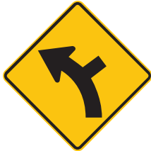
SIDE ROAD JUNCTION ON A CURVE
