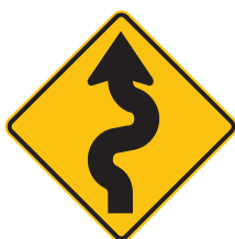
WINDING ROAD W1-5A W1-5B W1-5C
