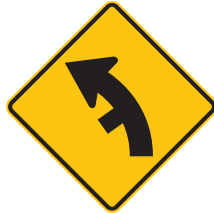
SIDE ROAD JUNCTION ON A CURVE
